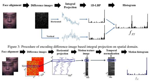
Figure 4: Motion histogram along horizontal direction: The blue rectangle represents the variation of horizontal projection at one position of Y-axis direction, where t and T are the original and temporal normalization time lengths, respectively.
