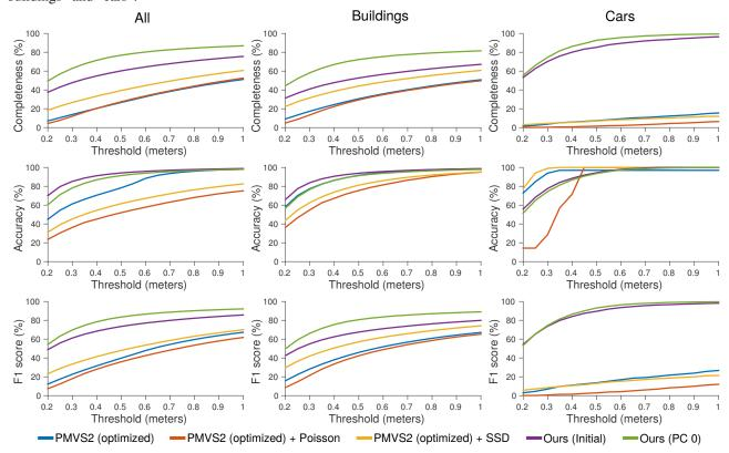
Figure 5: Varying the Evaluation Distance. This figure shows quantitative results in terms of completeness, accuracy and F1 score when varying the evaluation distance  $\tau$  between 0.2 and 1.0 m. To avoid clutter, we only show results for a subset of the methods. We refer the reader to the supplementary material for the full plots.
