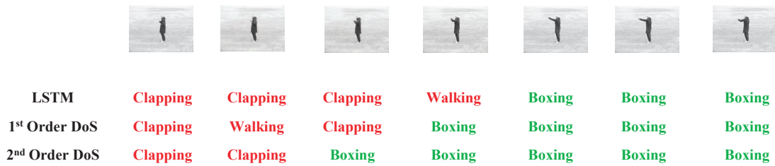
Figure 4. Frame-by-frame prediction of action category over time.
