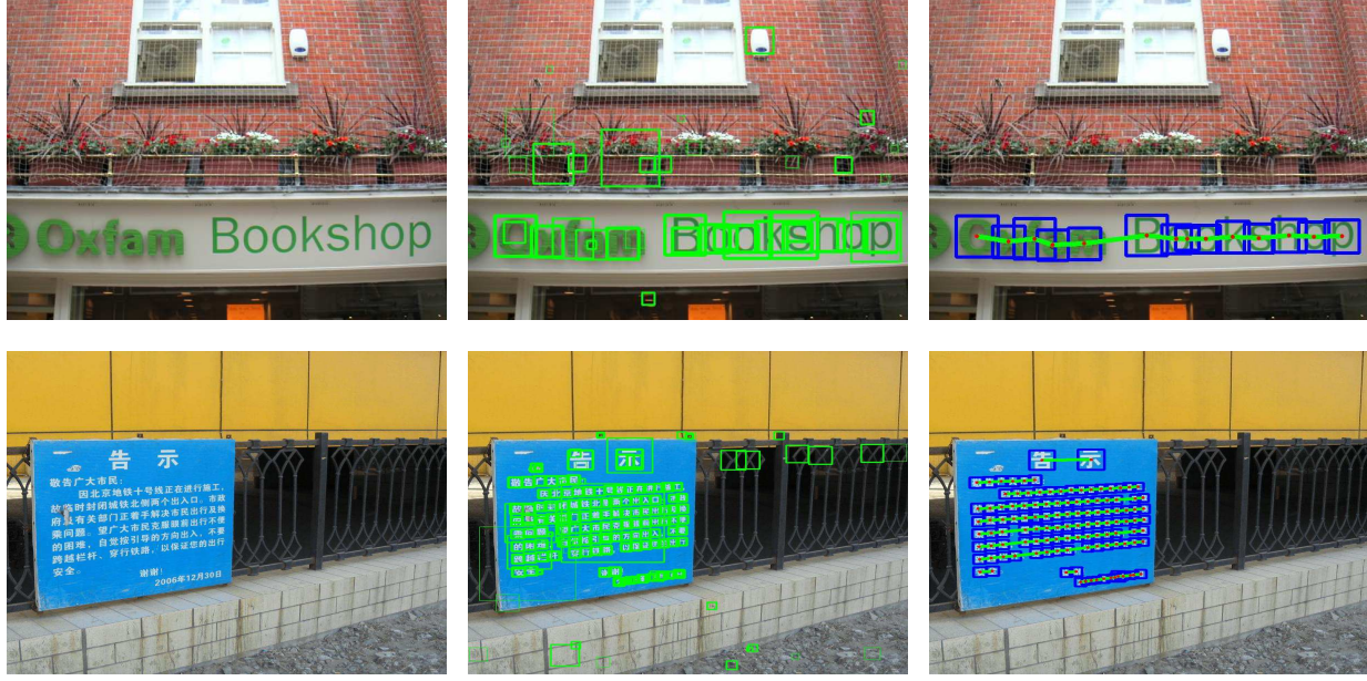
Figure 6: Illustration of text line extraction based on the min-cost flow network model: Input images are shown in the leftmost column and detected character candidates are labelled by green color bounding boxes as shown in the images in the middle column. The extracted text flows are labelled by green lines that link the identified true character (labeled by blue bounding boxes) as shown in the images in the rightmost column. The center of each identified true character is labelled by a red dot.
