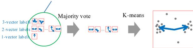
Figure 5. Prediction model by majority voting and K-means. In this sample,  $K = 2$ .
