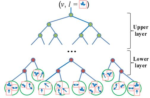
Figure 3. Training COUNT forest in a coarse-to-fine manner using two split layers. For space limit, only one tree is shown.
