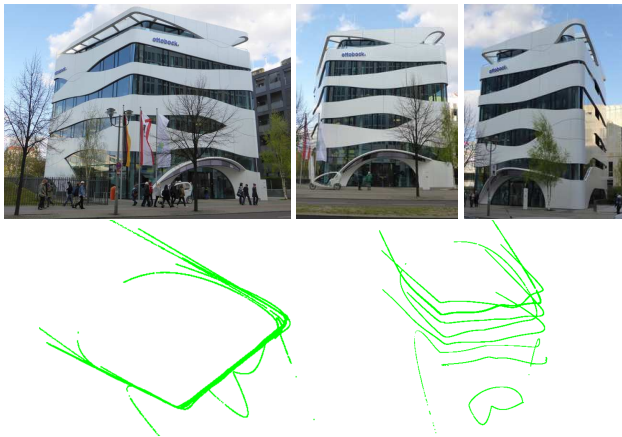
Figure 14: Three of ten views of a modern building (top). This is a very difficult case for curve-based matching as most of the curves are nearly parallel to epipolar lines. Our system produces a reasonable reconstruction of the curves (bottom), but does not significantly improve the camera estimates. Note that the building does actually have a rhomboidal floorplan.
