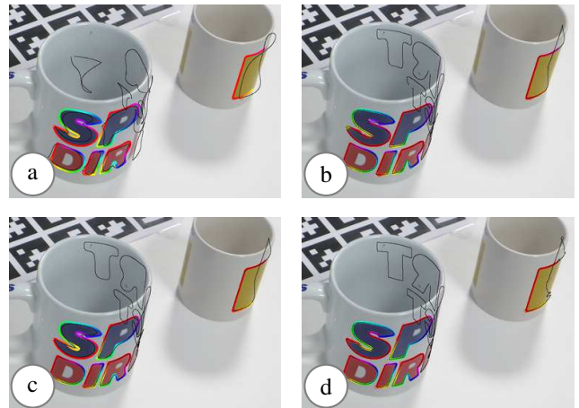
Figure 7: Curve refinement using dynamic programming. (a) Curve initialized using DP. (b) Final optimization result. (c) Reinitialized using optimized control points and cameras. (d) Final optimized curves. The fidelity of the complex curves (text) improves, but we begin to see overfitting on the simple rectangle. Future work will adaptively adjust the number of control points.
