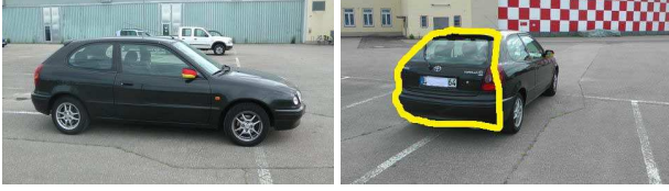
Figure 2. Changing viewpoints lead to disocclusion areas (marked) with content that was not visible in the original frame. It must be inferred if these regions belong to object or background.
