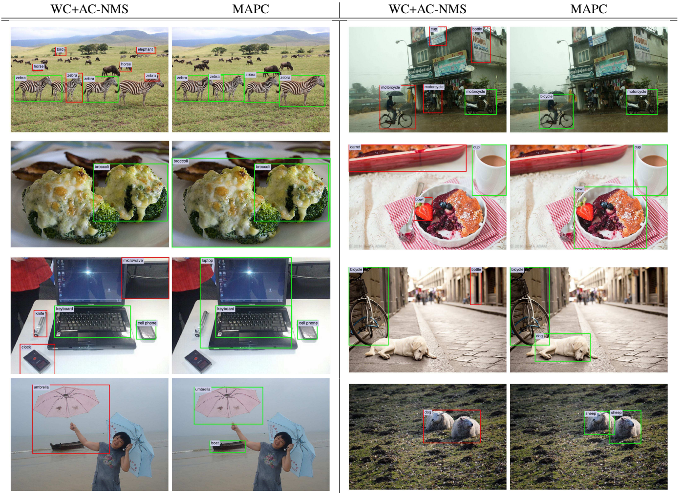
Figure 6. Examples, where MAPC outperforms WC+AC-NMS on Microsoft COCO. True positives: green, false positives: red.
