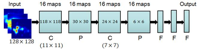
Figure 7. The structure of the Convolutional Neural Network (C: Convolutional Layer; P: Max pooling layer; F: Full connection layer). The CNN takes two ESMs ( $\mathbf{S}^1$  and  $\mathbf{S}^2$ ) and one GSM ( $\mathbf{G}$ ) as input, which are resized to the resolution of  $128 \times 128$ . A soft-max function is applied to the output of CNN so as to infer a binary label, which equals to 1 if  $\mathbf{S}^1$  outperforms  $\mathbf{S}^2$ , and 0 otherwise.
