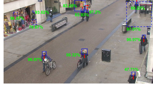
Figure 9. An example of head pose estimation result on the Towncentre dataset. Red arrows indicate the estimated direction. Its confidence score is written near the box. Dashed-line rectangles are the detections that are estimated as the background (i.e., false positive) by the proposed algorithm (see supplementary materials for more results).
