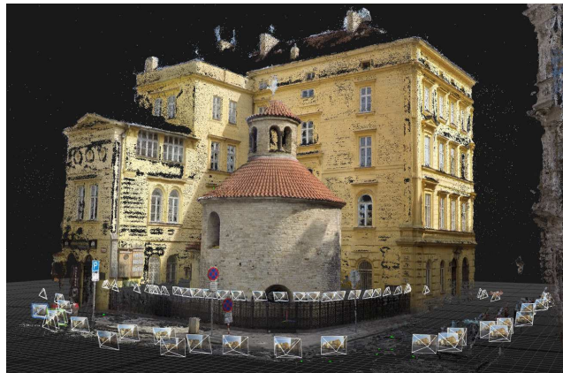
Figure 1: 3D Reconstruction of a rotunda captured by a GoPro Hero4 camera with varying field-of-view settings. The proposed F10 solver was used as a part of the SfM pipeline.
