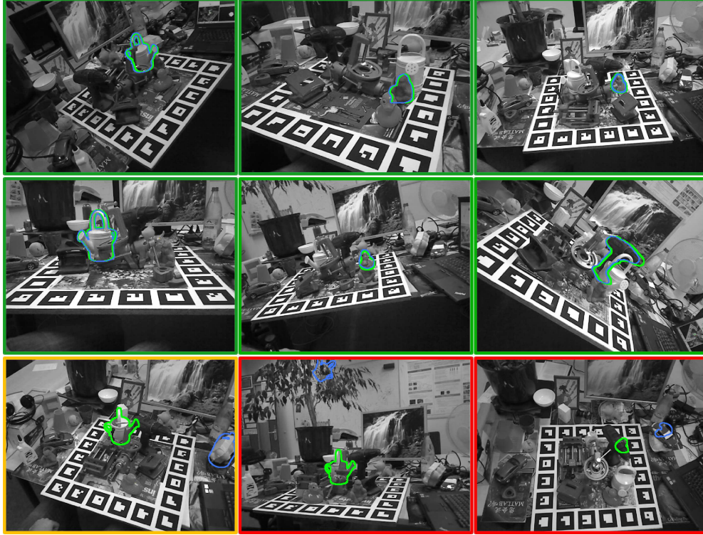
Figure 7. Qualitative results of our method on the occlusion dataset from [5] and [14]. Here, green and blue silhouettes correspond to the ground truth and our estimate, respectively. The test images depicted with a green frame show correct estimates. Images with orange and red frame show incorrect estimates. The image with an orange frame shows a case where the energy of the ground truth pose, according to Eq. (2), is lower than the energy of the estimated pose. In this case a better pose may be found with an improved optimization scheme.
