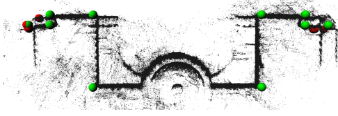
Figure 3. Connection points for sub-model 0 of the University dataset. Connection points resulting from the intersection of planes are colored in green, connection points created from the boundaries of planes are shown in red.
