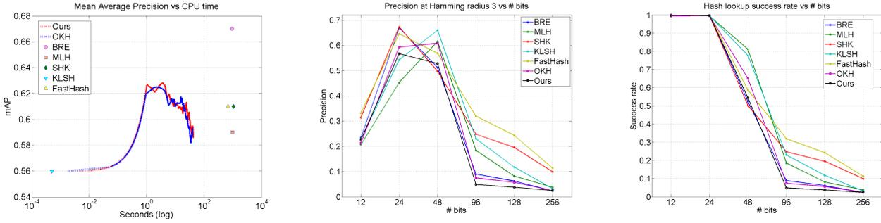
Figure 4: Results for the 22 LabelMe dataset. (Left) Mean Average Precision (at 96 bits) with respect to CPU time in which for OKH and our method, the online learning is continued for 10K pairs of points. (Center) Mean hash lookup precision with Hamming radius 3. (Right) Hash lookup success rate.
