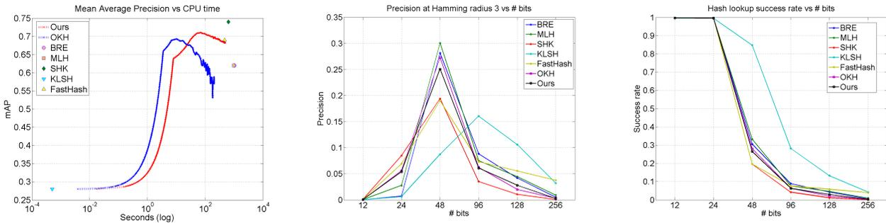
Figure 5: Results for the Halfdome dataset. (Left) Mean Average Precision (at 96 bits) with respect to CPU time in which for OKH and our method, the online learning is continued for 50K pairs of points. (Center) Mean hash lookup precision with Hamming radius 3. (Right) Hash lookup success rates.
