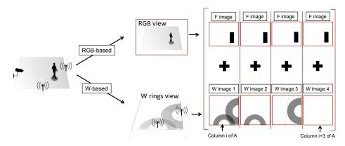
Figure 5: Illustration of dictionary construction given RGB-W data. For each ground plane point, the  $i^{th}$  column is made of the foreground ideal observation (F image) concatenated with the top view ring image of the W data for various antenna responses (W images i).
