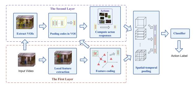
Figure 1. Illustration of the proposed two-layer structure on action classification. (Best viewed in color)
