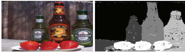
Figure 10. Stereo matching results of a deep outdoor scene. Left: one of the XSlit images acquired with slits of width 1\text{mm} . Right: our recovered disparity map.
