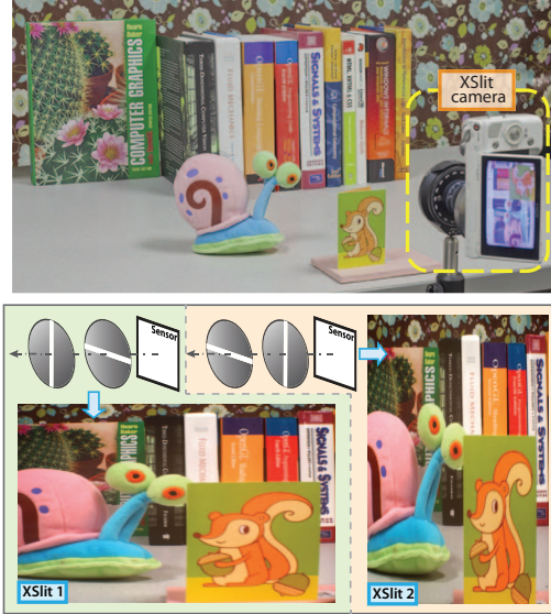
Figure 8. An R-POXSlit stereo pair of a study table scene captured by our prototype POXSlit camera.
