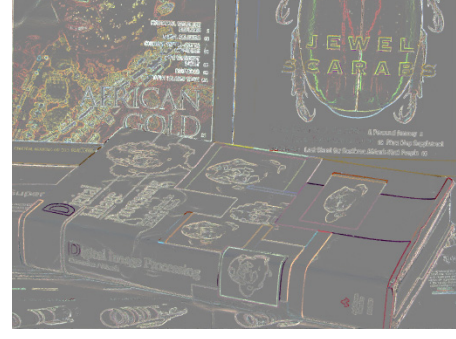
Figure 2. Optimal scale map s computed from images in Fig. 1 according to Eq. (1). Dark to bright pixels correspond to negative to positive values in different scales.
