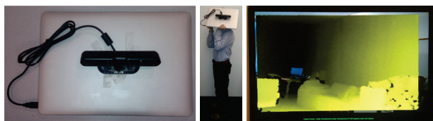
Figure 5. Data capturing setup . A operator carries an RGB-D sensor mounted on a laptop, mimicking natural exploration.
