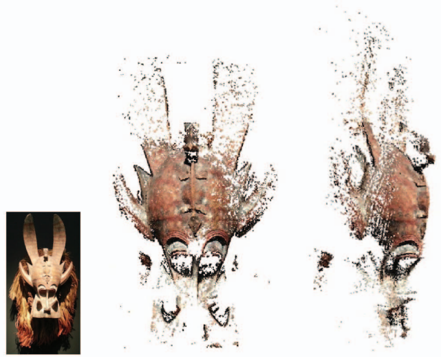
Figure 6. Photo and front and right view of the reconstructed 3D model of a 0.5 m tall African tribal mask.
