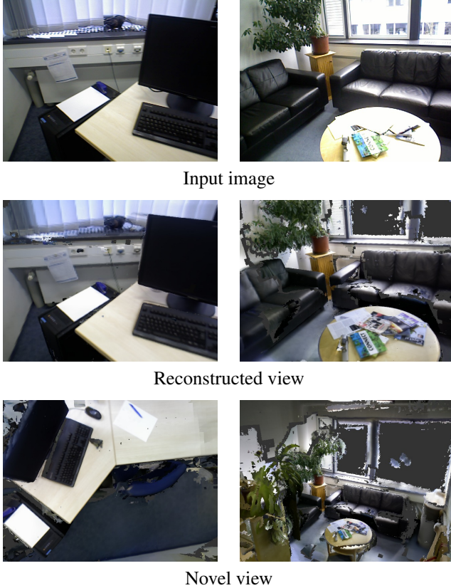
Figure 6: Sample reconstructions of two different sequences (left and right columns). Top row: Example input image. Middle row: Visualization of the 3D model from the same viewpoint. Bottom row: Visualization from a different viewpoint.
