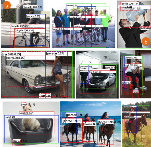
Figure 5. Object and visual composite detection: The central objects, object we want to re-score, are shown in red (only the top 3 detection responses are visualized), and the automatically discovered contextual objects in blue; green rectangles label the visual composites. For each detection response, we also show the confidence score before and after applying our relational model denoted by s : t , where s is the output of subcategory detector and t is the output of our full model. We use dashed line to denote the responses suppressed by our relational model, solid line for boosted responses. For example, in (a), a confident “person” score from 0.99 to 1.31 while the false positive bicycle response above the person is suppressed; (b) shows an example of “person-bottle” composite. Although the true positive bottle response is decreased, the gap between true positive and false positive bottles is increased.
