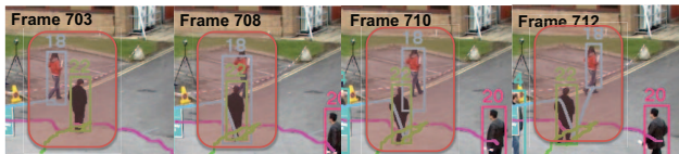
Figure 3. Instantaneous identity switch. In frame 703, targets 18 and 22 come close. Their bounding boxes overlap significantly in the frame 708 and their identities are momentarily switched. Afterwards, the targets separate and their identities are retained in frames 710 and 712.
