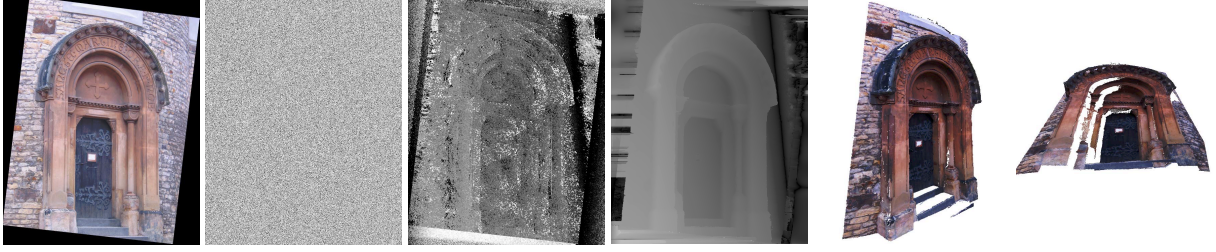
Figure 3: From left to right : One image of the portal stereo pair from [2], our disparity map after initialisation, disparity map after the 1st iteration, the final disparity map and two images with different views of a point-cloud generated using the final disparity map.
