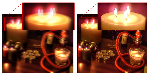
Exponential bracketing and conventional registration Fibonacci bracketing and generalized registration
