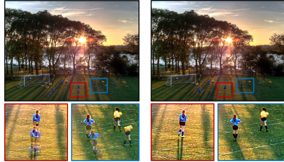
Fibonacci bracketing + Conventional registration Fibonacci bracketing + Generalized registration Figure 9. Comparison between conventional and generalized registration. The same LDR images (11 frames of a Fibonacci bracketing sequence) were used for both cases. Conventional registration does not exploit the iso-exposure property of Fibonacci bracketing. This results in incorrect registration and strong ghosting artifacts. Generalized registration produces a ghost-free image.
