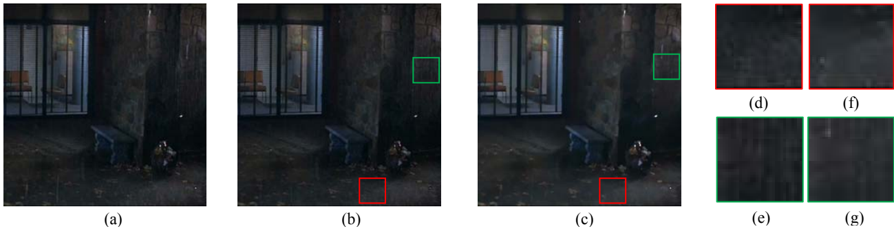
Figure 9: (a) A selected frame from video “forrest”; and the rain-removed results obtained by (b) [7]; and (c) our method. (d)-(e) and (f)-(g) show the enlarged red/green rectangles in (b)-(c), respectively.
