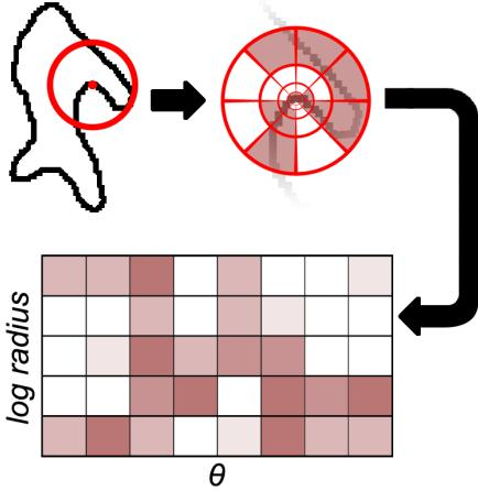
Figure 2: Example of shape context description on a human shape contour point using 5 radius bins and 8 angle bins.
