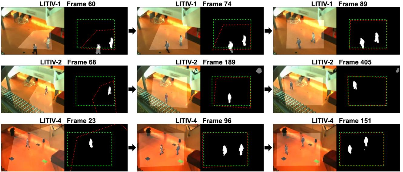
Figure 4: Registration results obtained at various moments of the first, second and fourth sequence pairs of the LITIV dataset using our proposed method. The left image in each pair shows the estimated frame-wide registration, and the right shows foreground shape registration at the same moment. The red dashed polygon shows the estimated transformation applied to the infrared image boundary, and the green one shows the ground truth transformation applied to this same boundary.
