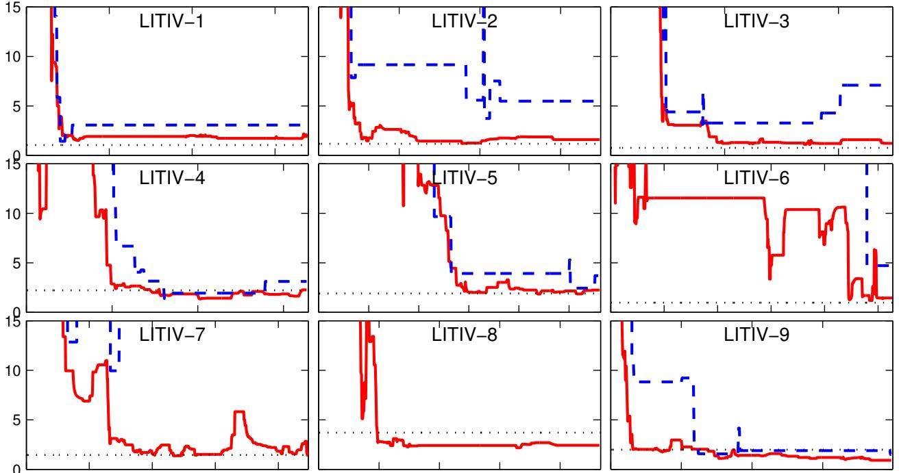
Figure 6: Polygon vertices Euclidean distance errors (in pixels) obtained using our method (solid red), the method of [19] (dashed blue), and the ground truth homography (dotted gray) for all sequences of the LITIV dataset. Note that the Y axis has been cropped similarly for all graphs.
