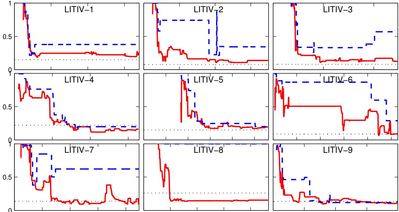
Figure 5: Polygon overlap errors obtained using our method (solid red), the method of [19] (dashed blue), and the ground truth homography (dotted gray) for the full lengths of all sequence pairs of the LITIV dataset.
