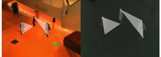
Figure 3: Example of the polygons used for quantitative evaluation formed with manually identified keypoints in the ninth sequence pair of the LITIV dataset.
