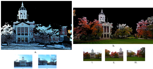
Figure 3. 2D-3D registration results. Fall and winter photographs registered with summer scan. Top : 3D environment after registration. Bottom : 2D images being registered.
