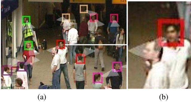
Figure 1. Image (a) illustrates an example from the PETS 2007 dataset [4] of our tracking output, the social groups (designated by colored bounding boxes) and the extracted gaze direction estimates (illustrated by field of view cones). image (b) is a zoomed subsection showing the gaze direction field of view of a person in the image.
