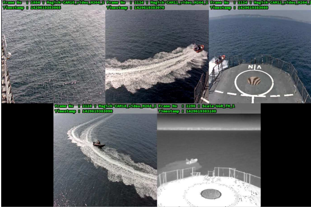
Figure 9. Example of synchronised images from IPATCH Dataset. Top row: Three visible cameras; Bottom row, left: visible camera. Bottom row, right: thermal camera.
