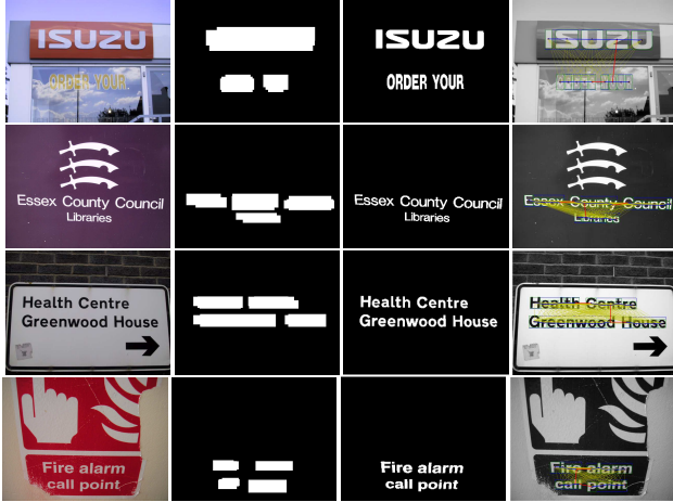
Figure 2: Detection Examples. From left-to-right inputs are shown followed by their results for: i) coarse detection, ii) fine detection and region growing, and iii) word segmentation. In word detection results, words are in blue boxes, and characters in green boxes. For simplicity, we represent word segmentation results using a Minimum Spanning Tree (MST) over character pairs (yellow lines) defining character merges (blue lines) and word separations (red lines). In actual fact, all character pairs are labeled as ‘merge’ or ‘split.’
