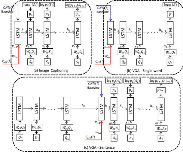
Figure 3. Language generators for different types of tasks: (a) Image Captioning, (b) VQA-single word, (c) VQA-sentence. red arrow indicates our attributes input  $V_{att}(I)$  while blue dash arrow shows the baseline method input  $CNN(I)$ .
