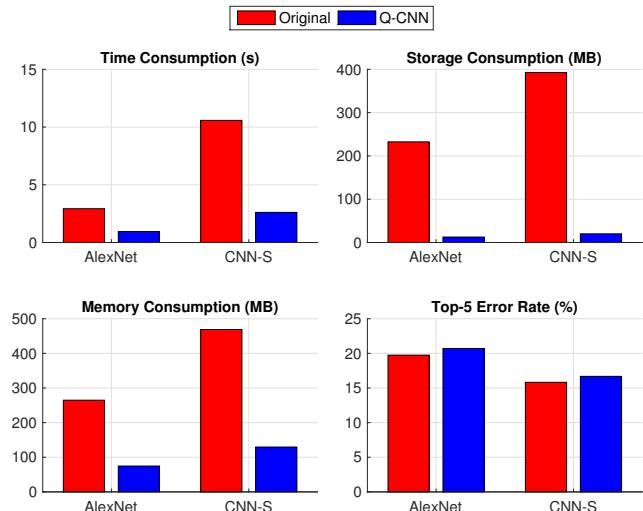
Figure 1. Comparison on the efficiency and classification accuracy between the original and quantized AlexNet [16] and CNN-S [1] on a Huawei® Mate 7 smartphone.
