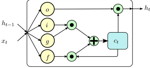
Figure 2. Schema of a long short-term memory (LSTM) unit.  $o$  is the output gate,  $i$  is the input gate,  $g$  is the input modulation gate, and  $f$  is the forget gate.  $c$  is the memory cell to keep the long term context.
