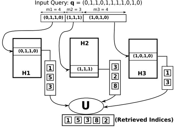
Figure 1. An illustration of the hashtable based retrieval mechanism given in Eq. 1. Here, the feature vector is split into 3 hashkeys of lengths  $m_1, m_2, m_3$  respectively. Each substring is a hashkey to the corresponding hashtables  $H_1, H_2, H_3$  respectively. Given a query vector  $\mathbf{q}$ , its substrings are used to retrieve relevant example indices before a final union to give the final retrieved indices.
