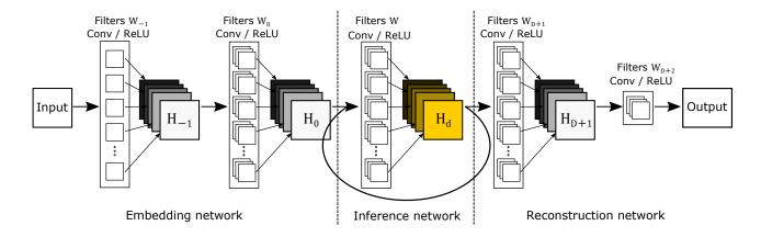
Figure 1: Architecture of our basic model. It consists of three parts: embedding network, inference network and reconstruction network. Inference network has a recursive layer and its unfolded version is in Figure 2.
