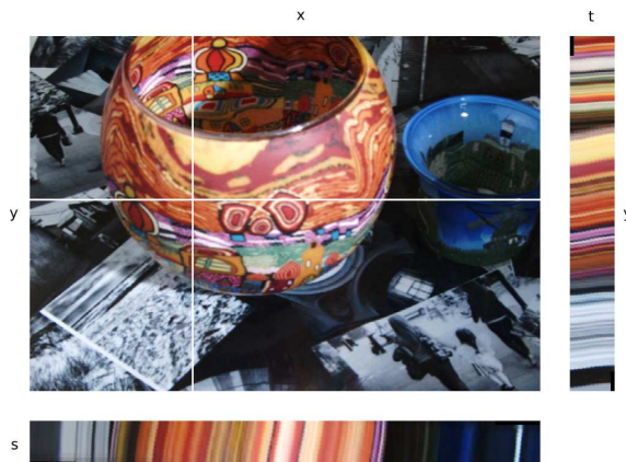
Figure 1. Epipolar plane images (EPIs) . The picture shows the center view of a light field parametrized by image coordinates x and y . On the bottom and right, the epipolar plane images for the white lines in the center view are shown, where s and t describe varying view point coordinates. As the camera moves, 3D scene points trace straight lines on the EPIs, whose slope is inversely proportional to the distance of the point [2]. Thus, orientation on the EPI is related to local depth.
