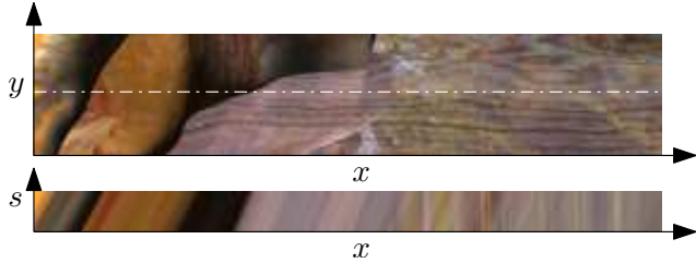
Figure 6. Light field with two disparity layers. The top image shows a close-up of the center view of the tiger dataset, see figure 5, courtesy of [29]. The EPI corresponding to the white line is depicted below. Parts of the surface are non-Lambertian and show a reflection, the corresponding regions of the EPI in turn exhibit two superimposed oriented patterns.
