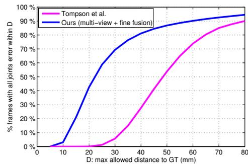
Figure 7: Comparison with the approach proposed in [29]. In this method, 14 hand joints are estimated. For fair comparison, in our method, 14 corresponding joints of 21 estimated joints are used to calculate the worst case accuracy.
