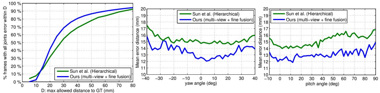
Figure 8: Comparison with the approach proposed in [21]. **Left:** the proportion of good test samples in the entire test samples over different error tolerances. **Middle & right:** the mean error distance over different yaw and pitch angles of the viewpoint. Our method holds smaller average errors in all of the yaw and pitch angles. The curves of the hierarchical regression method are cropped from the results reported in [21].
