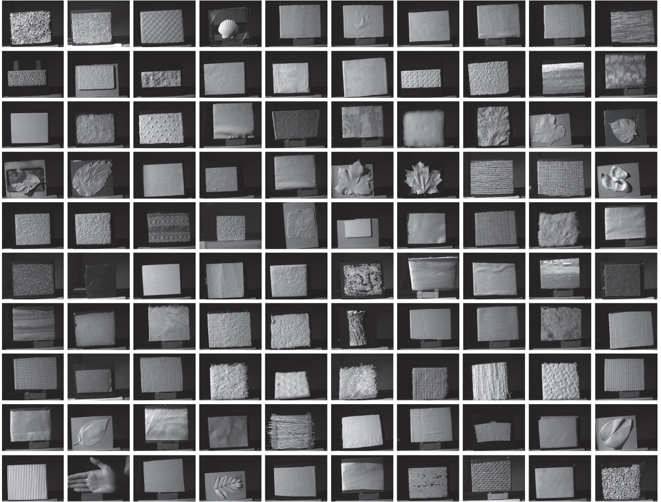
Figure 5. Our database consists of 100 real-world materials that include both natural and manmade and organic and inorganic samples. This is a superset of the materials in the original CURET database. Captured NIR images are shown. Full set of images under 12 lighting and 9 viewing angles, corresponding visible images and the BRDF and the surface detail models are available on-line. A complete listing of the materials is in the on-line web page.
