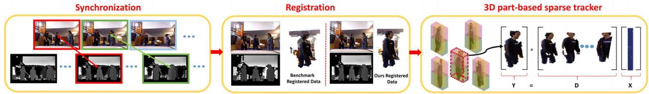
Figure 2. Overall pipeline for the proposed method, including the three major modules synchronization, registration, and 3D tracking.
