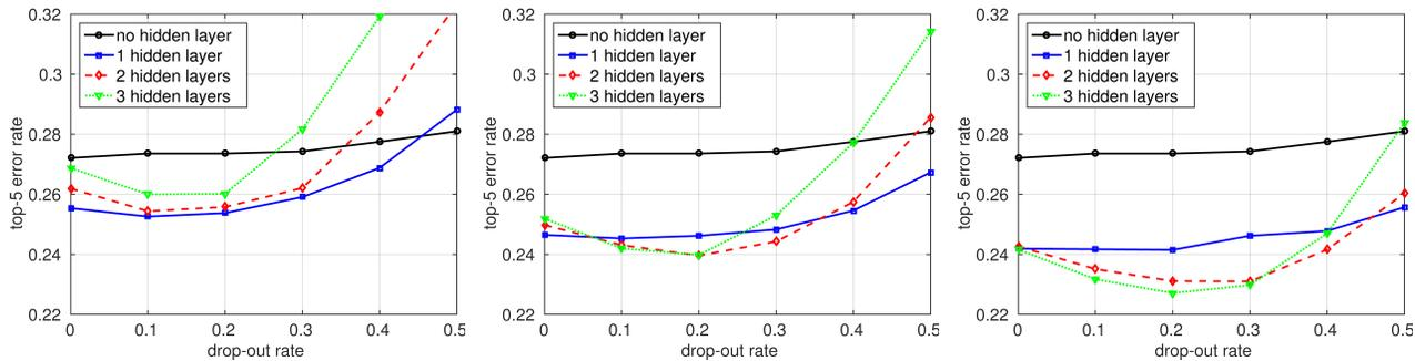
Figure 3. Top-5 error as a function of the drop-out rate for a variable number of hidden layers and a variable number of hidden units per layer: 1,024 (left), 2,048 (middle) and 4,096 (right) units per hidden layer (always the same number of units in each hidden layer).
