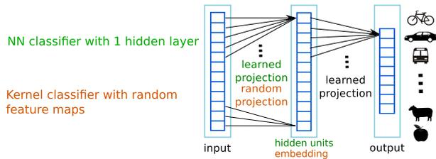
Figure 2. Comparison of a Neural Network classifier with a single hidden layer and a kernel classifier based on random feature maps.
