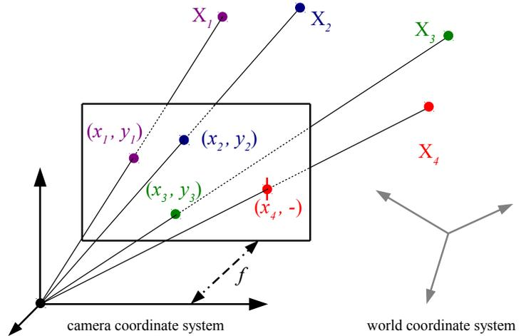
Figure 1: The P3.5P problem. The input are the 3 image points  $(x_1, y_1)$   $(x_2, y_2)$   $(x_3, y_3)$  plus either  $x_4$  or  $y_4$  of the 4-th image point and their corresponding 3D points  $\{X_1, X_2, X_3, X_4\}$  in the world coordinate system. The 7 image coordinates give sufficient constraints for this paper to recover the unknown focal length and camera pose.
