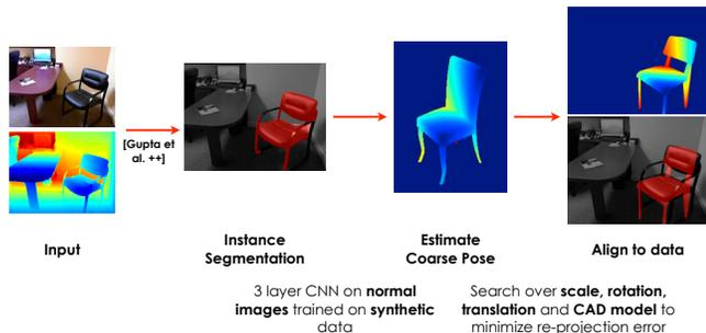
Figure 2: **Overview of approach:** We start with an improved version of the object detection instance segmentation output from [13]. We first infer the pose of the object using a convolutional neural network, and then search for the best fitting model that explains the data.
