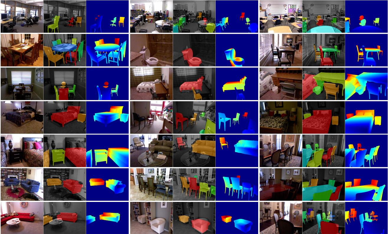
Figure 4: **Visualizations of the output on the test set:** We show images with multiple objects replaced with corresponding 3D CAD models. We show the image, models overlaid onto the image and the depth map for models placed in the scene. Depth maps are visualized using the ‘jet’ colormap, far away points are red and close by points are blue.
