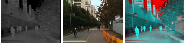
Figure 4. Image pairs captured by our hardware. (Left) thermal image. (Middle) color image. (Right) blending of the two images.
