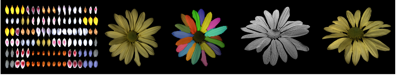
Figure 1. From left to right: 1) Petal database for Lily species; (2) Input image; (3) Petal segmentation; (4) Scanned 3D data; (5) Reconstructed 3D model.
