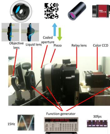
Figure 4. Setup of the camera.
