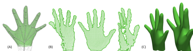
Figure 1: Hand shape fitting. (A) Template model with skeleton. (B) Three frames from 15-frame input sequence. (C) Template (left) and refined model (right) fit to this sequence. Note both a large scale change and local deformations (e.g. on the palm).
