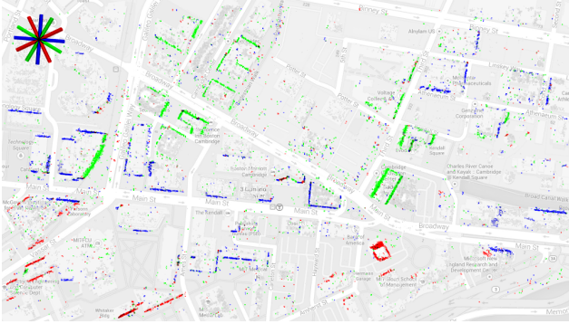
Figure 5: Inferred MMF from the LiDAR scanned urban scene on top of a gray street map. There is a clear separation into three MFs colored red, green and blue with the orientations indicated by the axes in the top-left corner. These MFs share the upward direction without imposing any constraints. Normals associated with upward axes are hidden to reveal the composition of the scene more clearly. Note that the underlying point cloud has varying density due to the scan-paths of the airplane.
