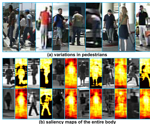
Figure 1. Pedestrian detection is challenging due to background clutter, poses, and large variations of appearance of the upper- and lower-body, as shown in (a). It is hard to learn a single model to represent each body part or the whole body. Background clutter also confuses detectors. SDN learns hierarchical features, saliency maps, and mixture representations of the entire body and different body parts. The saliency maps that separate the background clutters and the discriminative regions are shown in (b).
