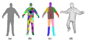
Figure 2. (a-c): reference model. (d): observations. (a) is a surface with  $N_v$  vertices. In (b) the surface is decomposed into  $N_p$  patches. (c) shows a rigged skeleton with  $N_j$  joints, and the associations between vertices and joints. (d) is a point cloud with  $N_y$  points. Typically,  $N_v \approx 4$ K,  $N_p \approx 150$ ,  $N_j = 15$ , and  $N_y \approx 9$ K.
