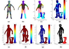
Figure 5. Comparison of outlier rejection in [12] (c-d) and ours (g-h). (a-b): reference surface colored in patches and body parts, respectively. (c): point cloud classified into body parts using the SVM trained on (b) from the previous frame, as suggested in [12]. (d): corresponding outlier likelihood from SVM. (e-f): two examples of Eq. 5. (g): point cloud colored based on Eq. 6. (h): points with outlier likelihood higher than 0.5 are colored in red.
