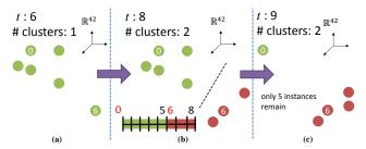
Figure 4. Illustration of Algorithm 2. (a): time frame t = 6,  $\mathcal{F} = \{0\}$ , and  $f_{\text{last}} = 0$ . (b): t = 8,  $\mathcal{F}$  becomes  $\{0, 6\}$ , and  $f_{\text{last}}$  becomes 6. (c): t = 9,  $\mathcal{F} = \{0, 6\}$ , and  $f_{\text{last}} = 6$ . Only 5 instances (9 - 6 + 2) are left for mean-shift.
